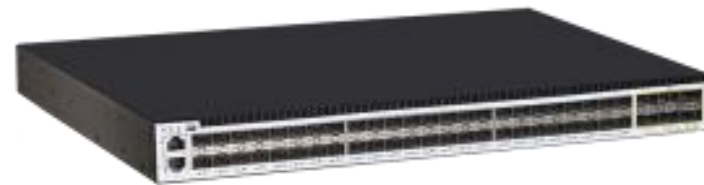
N10GSM6QF48 48 x SFP+ & 6x40GbE QSFP+ switch
