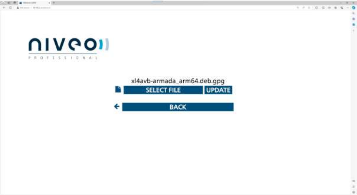
Screenshot 8: AVB update page of the webserver with update package being selected
