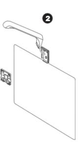
Slide Kaptivo unit onto mounting plate.
