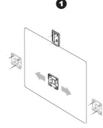
Install the rectangular Kaptivo mounting plate centered above board. Then install the square control pad mounting plate on your preferred side of the board. Use supplied screws. Maximum board size: 6 ft x 4 ft (1.8m x 1.2m)
