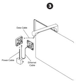
Wi-Fi Connection: Connect Kaptivo data cable and USB power cable to their respective sockets inside the control pad.
