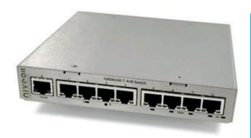
Niveo Professional introduces the brand new NGSME9AVB switch, offering a ready -out of the box- AVB switch that also supports Dante and PoE+. The switch requires no configuration or difficult firmware uploads, nor any payment or activation of AVB license fees.
